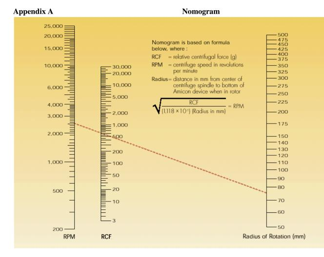
To convert RPM to relative centrifugal force (RCF): Determine centrifuge's radius of rotation (in mm) by measuring distance from center of centrifuge spindle to bottom of device when inserted into rotor. Lay a ruler and draw a line from radius value in right-hand column to 1500 RCF in the middle column and continue the line to the RPM column on the left. Then read the RPM value from column at left. This is the value you will enter into your centrifuge to equal 1500 RCF (G-force).
